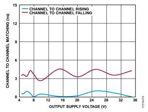
Figure 19. Channel to Channel Matching vs. Output Supply Voltage, Rising and Falling
