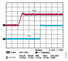
Figure 8. Typical  $V_{DD1}$  Delay to Output Waveform,  $V_{Ix} = V_{DD1}$
