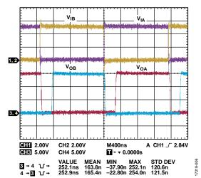
Figure 6. Dead Time Operation Between Input and Output with 50 k $\Omega$ Dead Time Resistor
