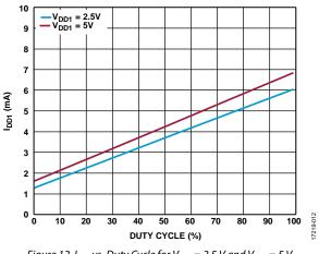
Figure 12.  $I_{DD1}$  vs. Duty Cycle for  $V_{DD1} = 2.5$  V and  $V_{DD1} = 5$  V,  $V_{DD2} = 15$  V ( $V_{DD2}$  Refers to  $V_{DDA}$  or  $V_{DDB}$ )
