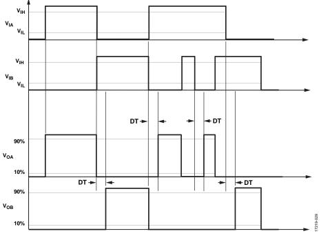
Figure 29. Dead Time Operation for Different Input Transitions
