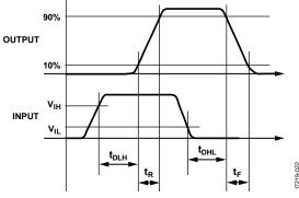
Figure 26. Propagation Delay Parameters
