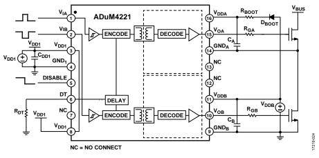
Figure 30. Circuit of Bootstrapped Half Bridge Operation
