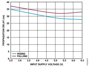
Figure 17. Propagation Delay vs. Input Supply Voltage, Rising and Falling,  $V_{DD2} = 15 V (V_{DD2} \text{ Refers to } V_{DDA} \text{ or } V_{DDB})$
