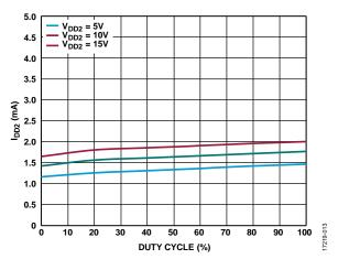
Figure 13.  $I_{DD2}$  vs. Duty Cycle for  $V_{DD2} = 5 V$ ,  $V_{DD2} = 10 V$ , and  $V_{DD2} = 15 V$ ,  $V_{DD1} = 5 V (V_{DD2} Refers to V_{DDA} or V_{DDB})$
