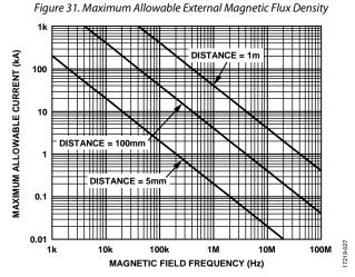
Figure 32. Maximum Allowable Current for Various Current to ADuM4221 Spacings
