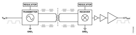
Figure 24. Operational Block Diagram of OOK Encoding (V<sub>IN</sub> Is the Input Voltage, and V<sub>OUT</sub> Is the Output Voltage.)
