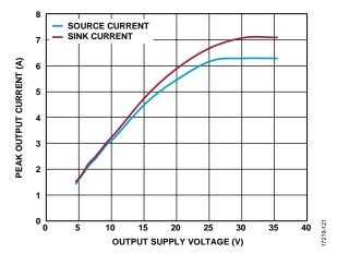
Figure 21. Peak Output Current vs. Output Supply Voltage with a  $2.2 \Omega$ Series Gain Resistor
