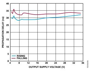
Figure 18. Propagation Delay vs. Output Supply Voltage, Rising and Falling, V<sub>DD1</sub> = 5 V
