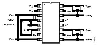
Figure 25. Recommended PCB Layout
