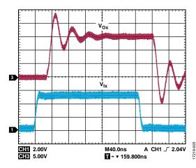
Figure 5. Output Waveform for 2 nF Load and 0  $\Omega$  Series Gate Resistor with 15 V Output Supply
