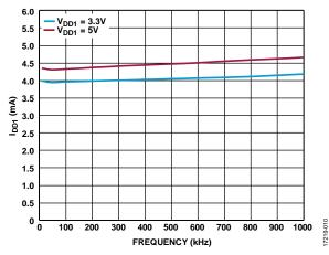
Figure 10.  $V_{DD1}$  Current ( $I_{DD1}$ ) vs. Frequency for  $V_{DD1} = 3.3$  V and  $V_{DD1} = 5$  V, 50% Duty Cycle
