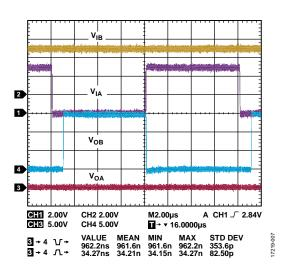
Figure 7. Dead Time Operation Between Input and Output with 200 k  $\Omega$  Dead Time Resistor and One Input Held High
