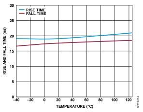
Figure 14. Rise and Fall Time vs. Temperature with a 3.9 Ω Series Gate Resistor for a 2 nF Load and a 15 V Output Supply
