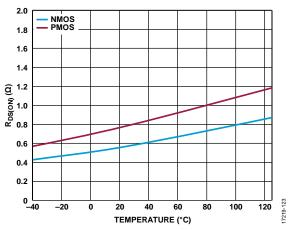
Figure 23. R<sub>DS(ON)</sub> vs. Temperature for NMOS and PMOS
