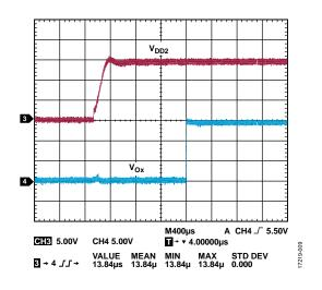
Figure 9. Typical  $V_{DD2}$  Delay to Output Waveform,  $V_{lx} = V_{DD1}$ ( $V_{DD2}$  Refers to  $V_{DDA}$  or  $V_{DDB}$ )
