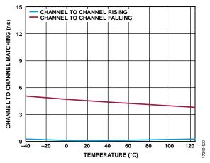
Figure 20. Channel to Channel Matching vs. Temperature, Rising and Falling, V<sub>DD2</sub> = 15 V (V<sub>DD2</sub> Refers to V<sub>DDA</sub> or V<sub>DDB</sub>)
