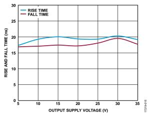
Figure 15. Rise and Fall Time vs. Output Supply Voltage with a 3.9  $\Omega$  Series Gate Resistor for a 2 nF Load
